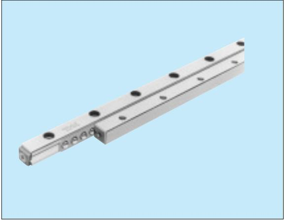
Low-friction, high-precision LM system. The ball cage, in which precision steel balls are arranged at a short pitch, moves among the V-groove machined on the rail, over only half the full stroke.
