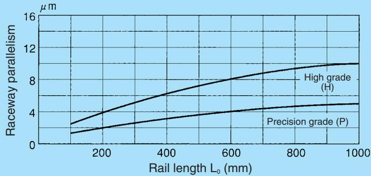
Fig. 3 Rail Length and Raceway Parallelism
