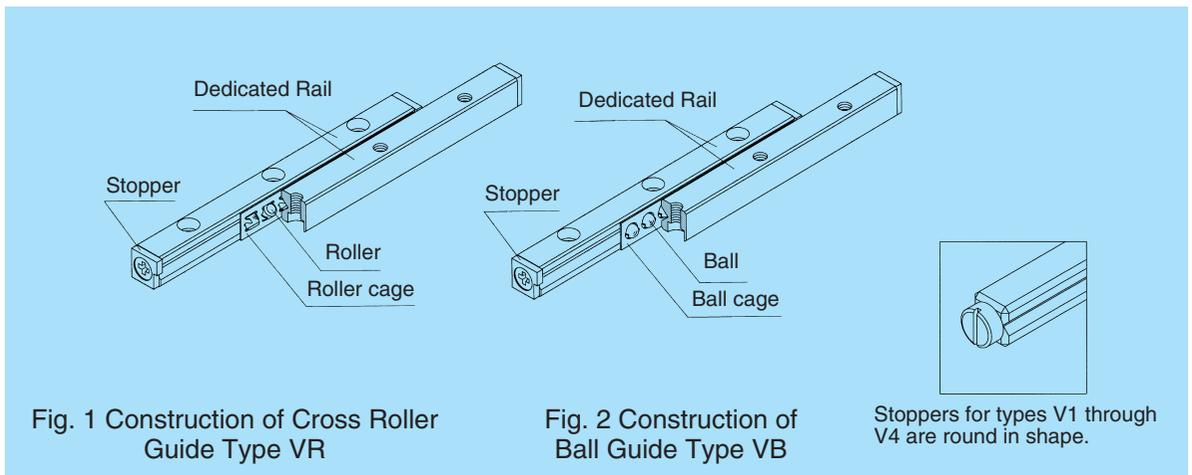
Fig. 1 Construction of Cross Roller Guide Type VR
